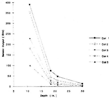
**Figure 15: Different Coils Output Data for Various Burial Depths**
