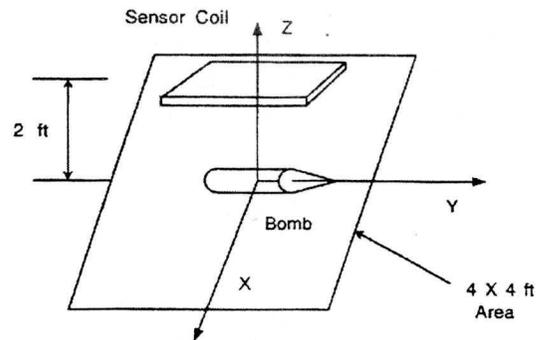
**Figure 18: Field Test Setup Using Coil 3 With Ordnance Parallel to Y-Axis and Parallel to the Horizontal Plane**
