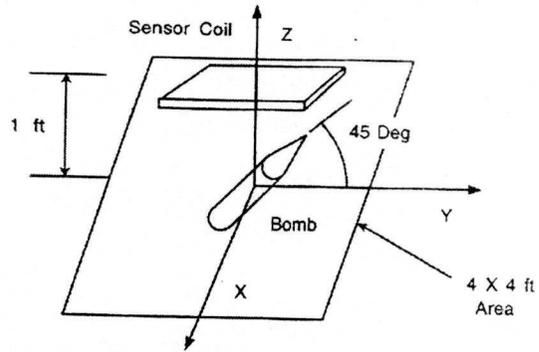
**Figure 21: Field Setup Using Coil 3 With Ordnance Parallel to Y-Axis and 45 Degrees to the Horizontal Plane**
