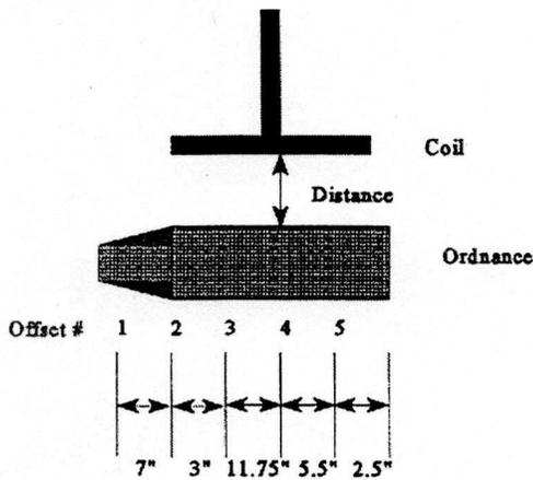
**Figure 23: Configuration and Definition of Offsets**
