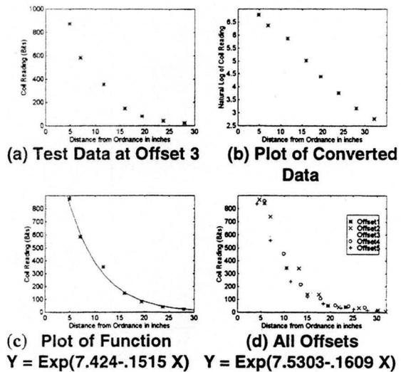
**Figure 24: Analysis of Test Data at Offset 3**
