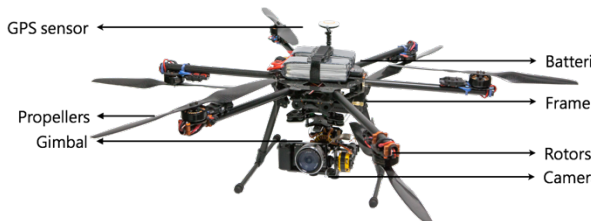
Figure 2. A typical six-propeller UAV consists of a frame, six rotors, propellers, batteries, and measuring equipment [7].
