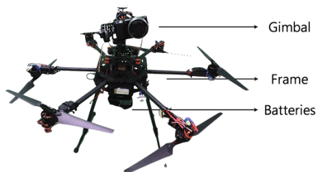
Figure 3. The improved UAV for a bridge inspection has the camera installed on top of its frame.
