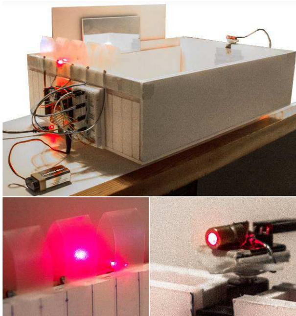
Figure 6. *Top*: Scaled-model of the AAL apartment at BR<sup>2</sup>'s Robotics Lab. *Bottom-left*: Module B's LSR 2 detecting a significant laser incidence. *Bottom-right*: Module A's laser component.
