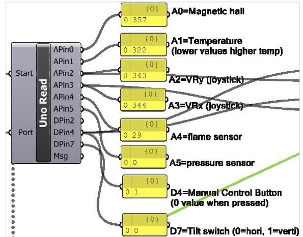
Figure 5. Sensed-data from Module A (in *McNeel's Rhino 5.0* & the plug-ins *Grasshopper* + *Firefly*).
