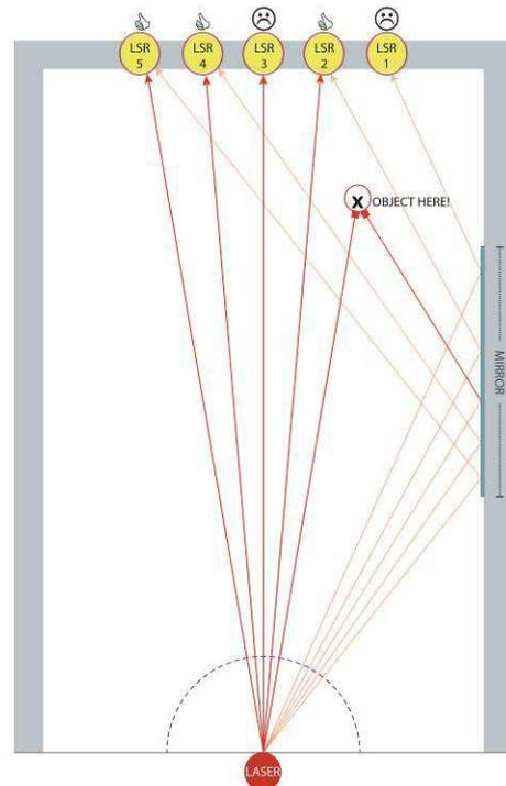
Figure 10. Finding the obstructing object with LSR 1's direct and LSR 3's indirect (i.e., reflected) lines of sight.
