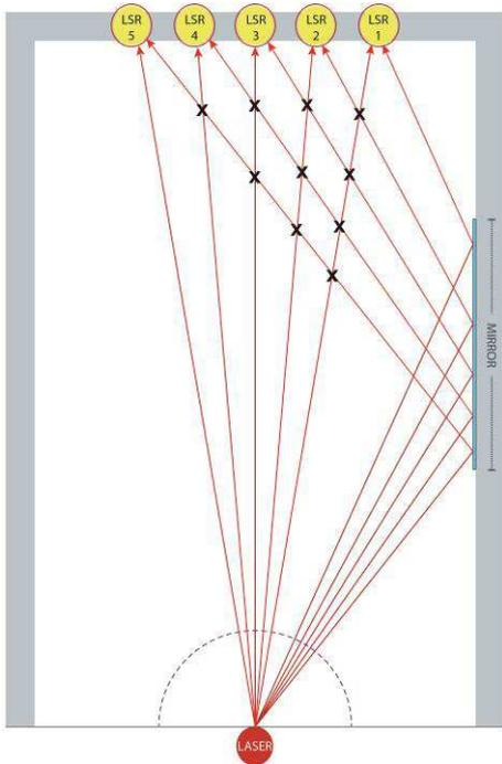
Figure 8. Conceptual illustration of scaled-model using Pyo *et al.*'s [21] proposed method. Xs indicate theoretical intersections.
