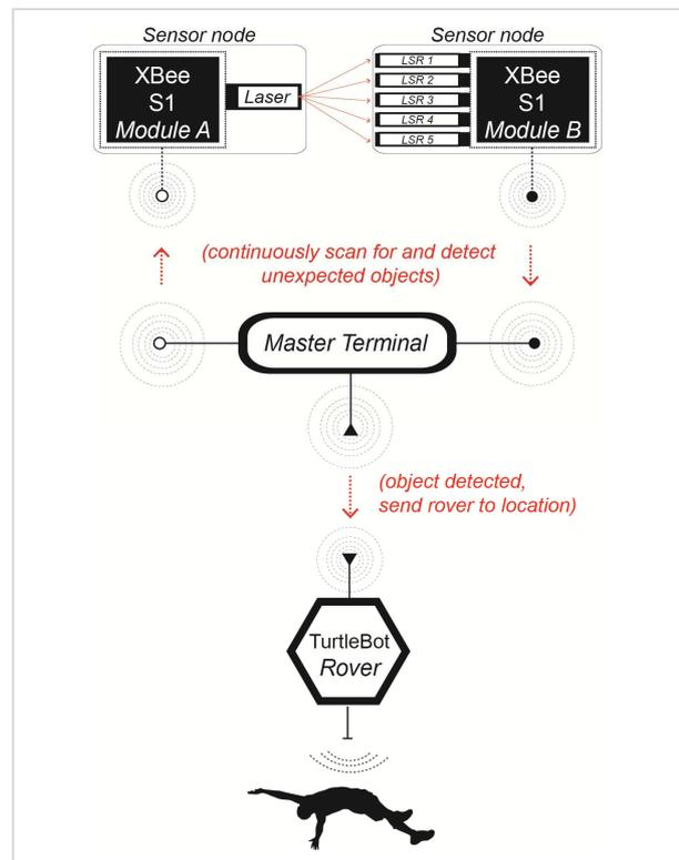
Figure 1. Diagram of overall concept.
