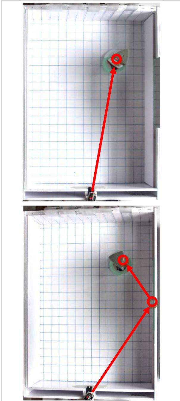
Figure 12. Physical scaled-model version of Figure 10. *Top*: Object blocking LSR 1's direct line of sight. *Bottom*: Object blocking LSR 3's indirect (i.e., reflected) line of sight.
