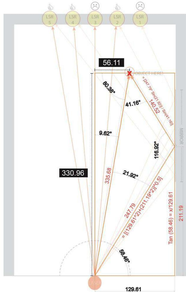
Figure 13. Calculations to find the planar position of the obstructing object (scaled-model units in millimeters).
