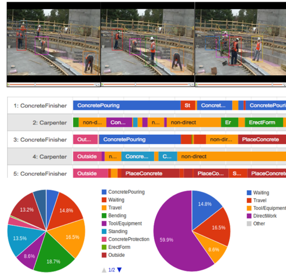
Figure 2. The Task Management interface: (top) annotated video; (middle) crew-balance chart; and (bottom) detailed and CII-type activity pie charts. The annotations in the upper left corner of each box overlaid on the annotated video shows the role-activity-tool-body posture of each worker.
