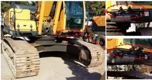
Figure 8. Stereo camera system mounted on an excavator
