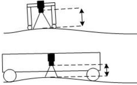
Figure 7. Height of sensor camera on AGV is variable on a corrugated surface
