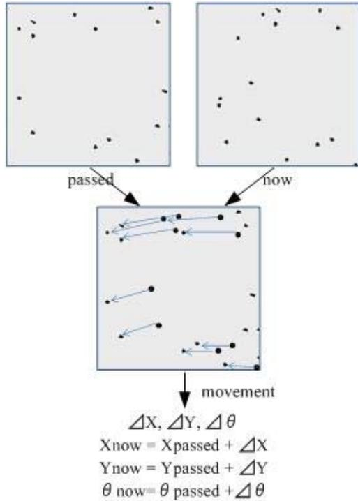
Figure 3. Detecting Movement Method
