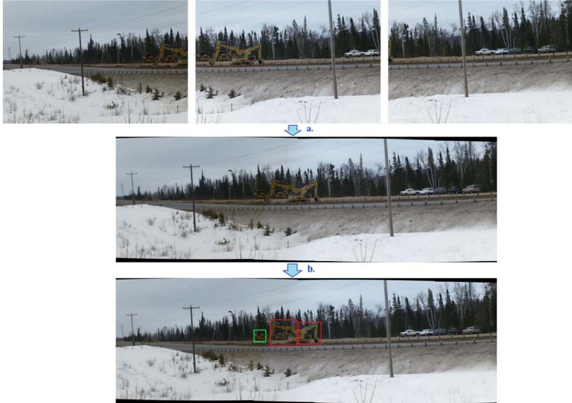
Figure 2. Steering of a PTZ camera to locate operations: a) stitching of images to create a panorama, b) object detection
