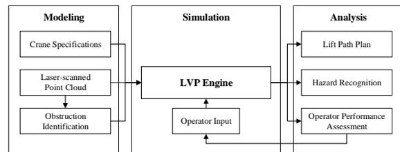
Figure 1: Framework of the Lift Virtual Prototyping (LVP) approach
