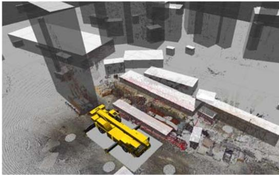
Figure 2: Reconstructed virtual lift scenario with laser scanned point cloud and bounding boxes generated for identified obstructions.
