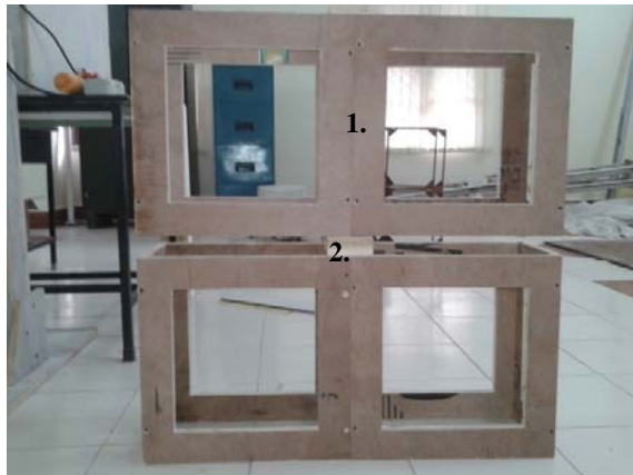
Figure 3: Lock for interlocking. The space between the flanges of the lock hold together the web of adjacent modules.
