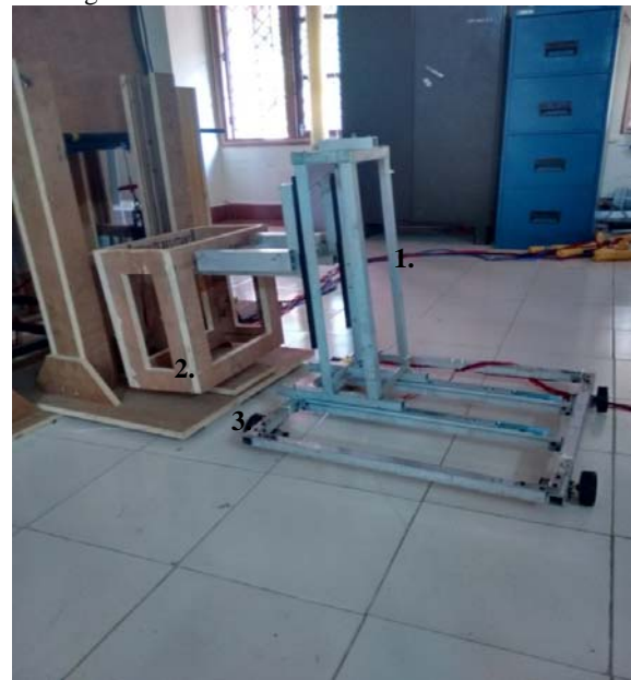
Figure 7: Robot for aligning modules; 1. Robot; 2. Module; 3. Lifting Module
