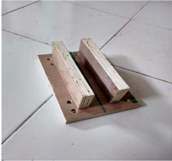
Figure 3: Lock for interlocking. The space between the flanges of the lock hold together the web of adjacent modules.
