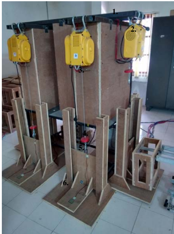
Figure 5: Lifting module and Actuator; 1. Metal Frame; 2. Actuator; 3. Steel Rope; 4. Metal Hook; 5. Lifting Module; 6. Load cell sensor
