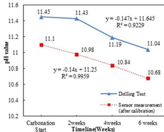
Figure 6. pH value comparison between sensor measurement and drilling test after calibration
