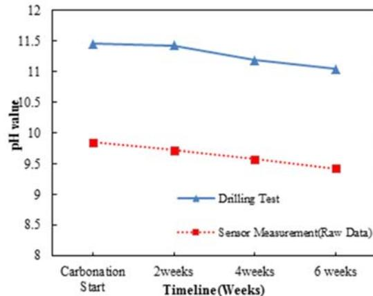
Figure 4. Comparison of 6 weeks carbonation value from raw pH sensor readings and drilling test
