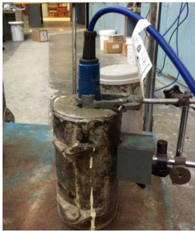
Figure 2. set-up of pH sensor embedment
