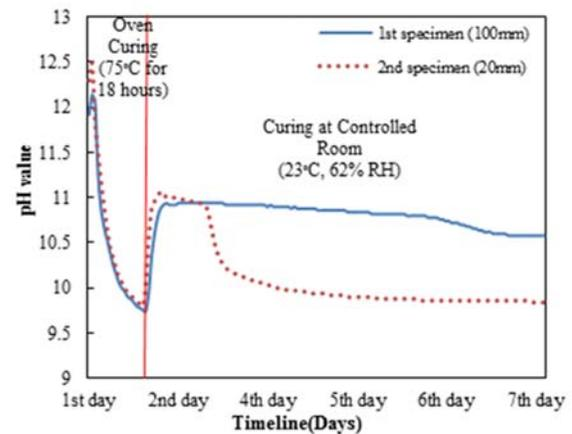
Figure 3. pH value during the heat and normal curing process
