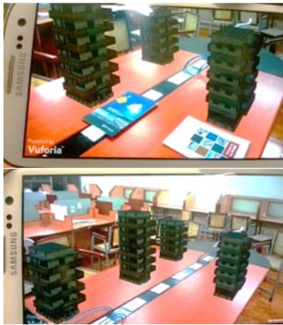
Figure 3. Models in place even after respective image targets have been removed. This is made possible by enabling extended tracking feature.
