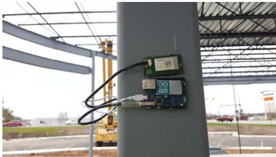
Figure 6. Steel component tagged with Swarm Node
