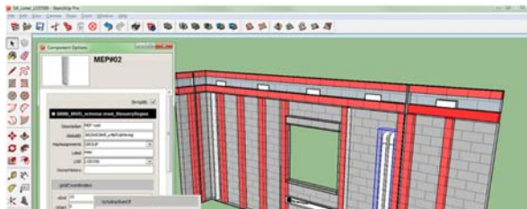
Figure 6 Masonry cavity wall modeled in SketchUp at LOD 350. Regions are created by top-down decomposition and assigned to predefined feature types by means of the “ isAbstractionOf ” relation. In this example the region represents CMU blocks in the back-up wall containing MEP ductwork.
