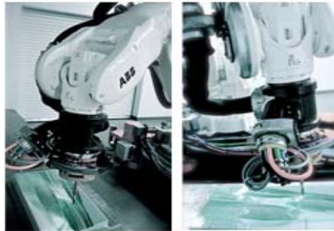
Figure 11. Physical prototyping – real-time workflow synchronized with virtual model.
