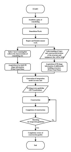
Figure 4. Remodeling construction process considering as-built
