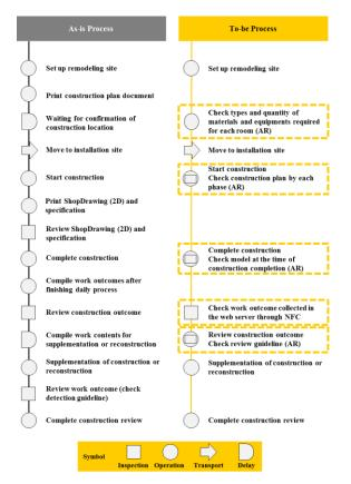
Figure 6. Augmented reality based review of construction quality process chart
