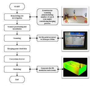
Figure 3. Laser Scanning process that reflects the remodeling characteristics [10]
