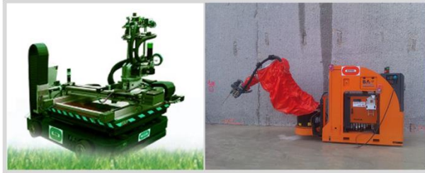
Figure 6. Existing drilling STCR developed in France by general contractor Bouygues Construction.
