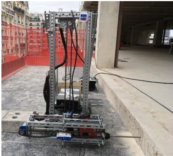
Figure 1. Picture of the drilling robot prototype
