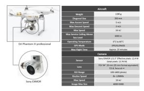
Figure 2. UAV and Camera
