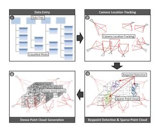
Figure 1. .Input 2D image, Calculation of camera pose, Generation of 3D point-cloud
