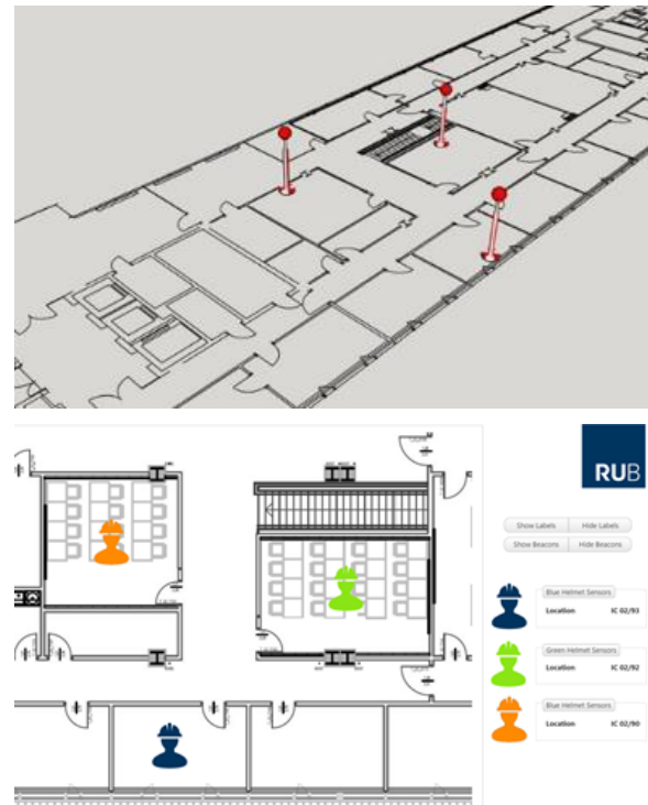
Figure 7. BLE-beacon positions planned in BIM (top) and real-time work station occupancy visualization by trade (bottom)
