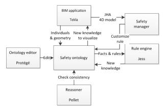
Figure 2. System architecture of the ontology-based hazard identification application in BIM
