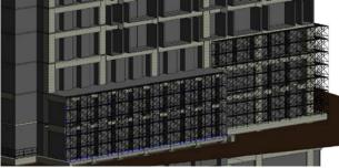
Figure11. Automated planning of scaffolding system
