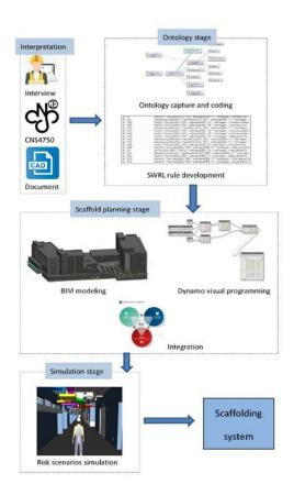
Figure 4. A framework of using BIM to automate scaffolding planning for risk analysis
