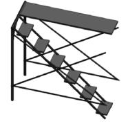
Figure 9. Self-made scaffolding BIM element
