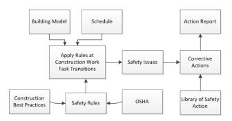
Figure 1. A framework for implementing an automated rule-based safety checking in BIM
