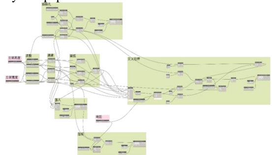
Figure 6. Dynamo module of scaffolding components
