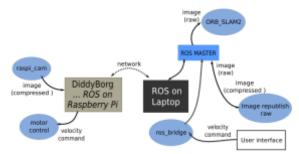
Figure 2: An example of the relationships of different nodes. The route the velocity commands and image data takes between the robot and the relevant node is also shown.
