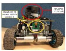
Figure 1: A photo of the DiddyBorg robotic platform with the locations of the RPLIDAR and Raspberry Pi camera sensors used in this work.
