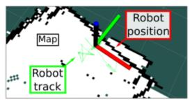
Figure 7: Shows the result of hector\_slam with the robot position and path marked by in the figure. Localisation and mapping errors occur in this example because the RPLIDAR is tilted out of its original plan without any update e.g., using data from an IMU.
