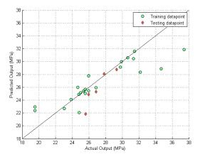
Figure 5. Actual and predicted concrete strength by SOS-SVR prediction model at training and testing stages for one fold (14-day strength test result).
