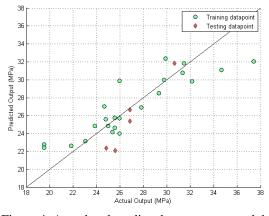
Figure 4. Actual and predicted concrete strength by SOS-SVR prediction model at training and testing stages for one fold (7-day strength test result).
