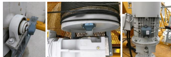
Figure 7: Implementation of Lora-tags on tower crane motors (i.e., raise/lower, move in/outwards, turn)
