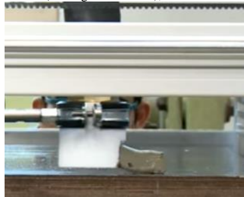
Fig. 4: Concrete technological extrusion trials on a scale of 1:5
