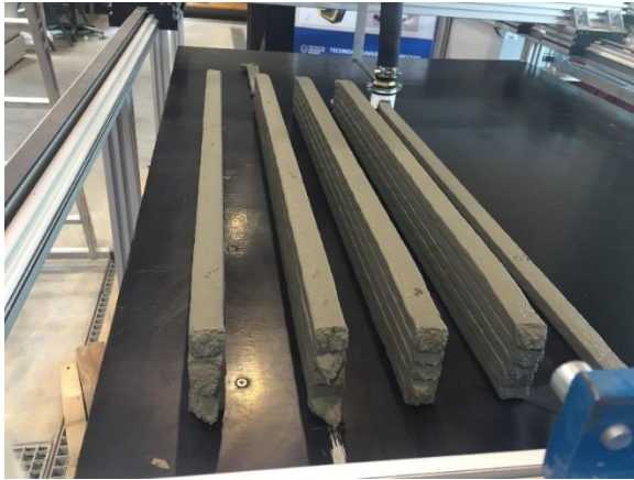
Fig. 5: Printed concrete components for the investigation of the layer composite
