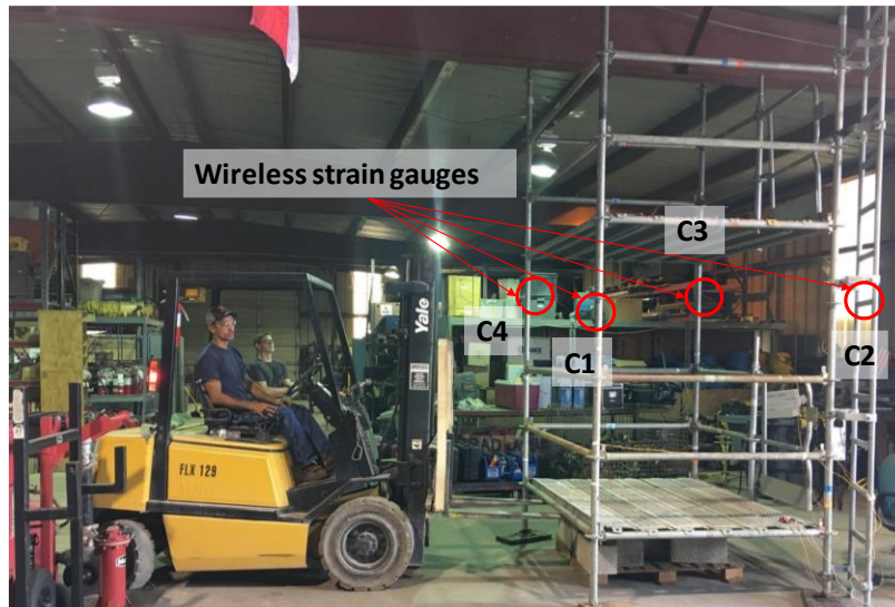
Figure 7 Experimental setup for uneven settlement and overturning conditions
