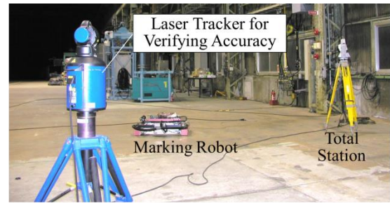
(a) Overall view of the test
