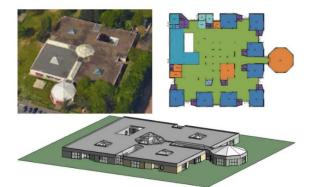
Figure 4. Aerial view of the kindergarten "H.C. Andersen", floor area with functional spaces and BIM model.
