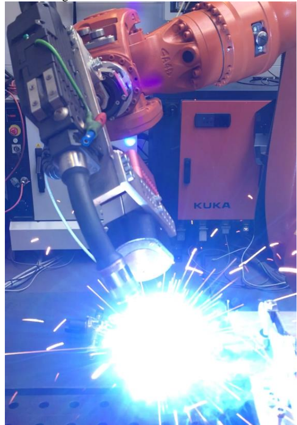
Figure 1 Robotic Incremental Point Welding
