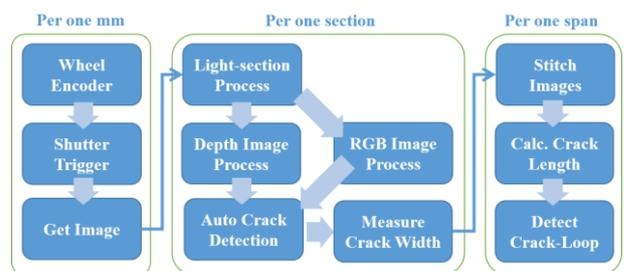
Figure 2. Crack inspection flow by our device
