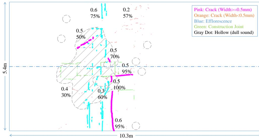
Figure 9. Inspection result by our method with crack width and crack detection rate
