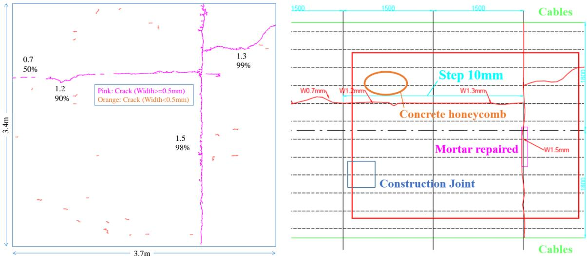
Figure 12. Crack inspection result with crack width and detection rate (L: by our method, R: by experts)
