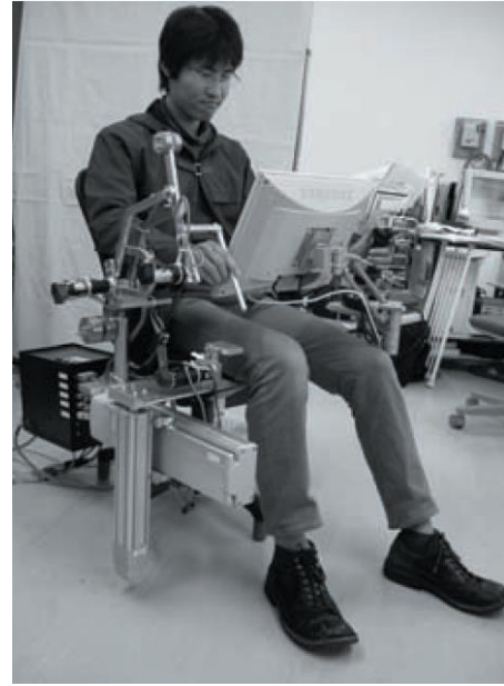
Figure 6. The operation system with force feedback controller [3]
