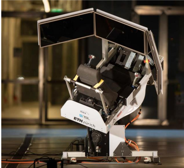
Figure 5. Moving operation seat for the remote control system [2]
