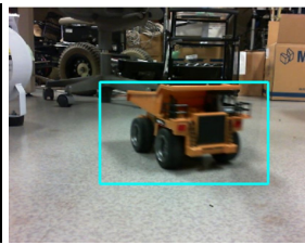
Figure 4. The result of moving object detection by background subtraction
