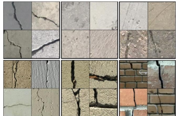
Figure 2. Training and test image samples. Positive training samples (top left), Negative training samples (top center), Possible false-positive training samples (top right), Concrete test samples (bottom left), Pavement test samples (bottom center), Brickwork test samples (bottom right)
