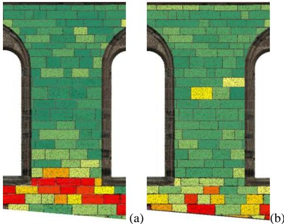
Figure 3. Geometry- and colour-based parameters (a)  $Ra$  (b)  $H_{\sigma}$
