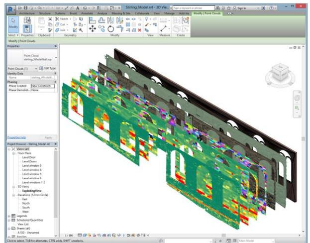
Figure 11. Datasets attached to the HBIM model
