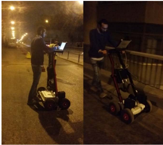
Figure 3: GPR data collection for El-Kobba bridge deck
