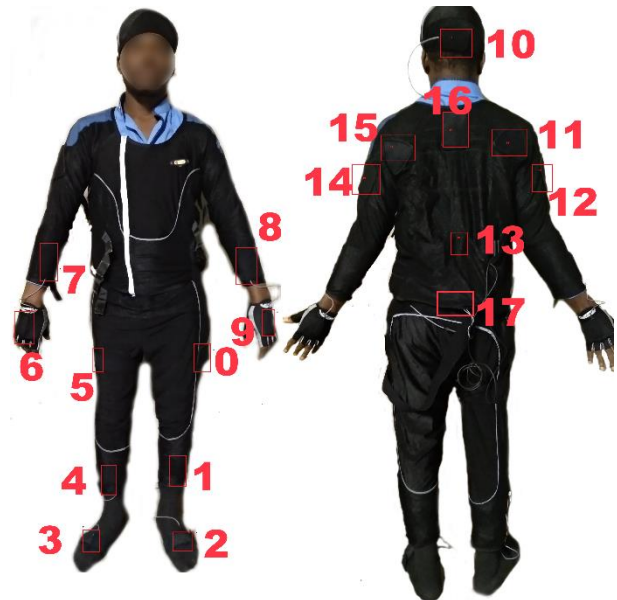
Figure 4. Inertia 3DSuit infrastructure showing the location of the IMU sensors.
