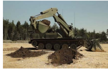
Fig. 4: Teleoperated trench digging [88].
