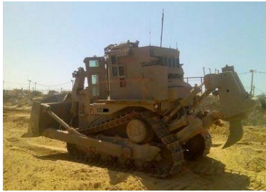
Fig. 6: Robotic bulldozer used by Israel Defence Forces [90].
