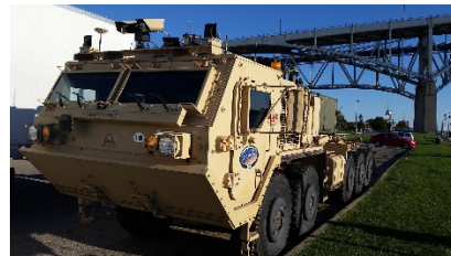
Fig. 5: The US Army is testing a "leader-follower" system that will employ up to 8 convoy vehicles [89].
