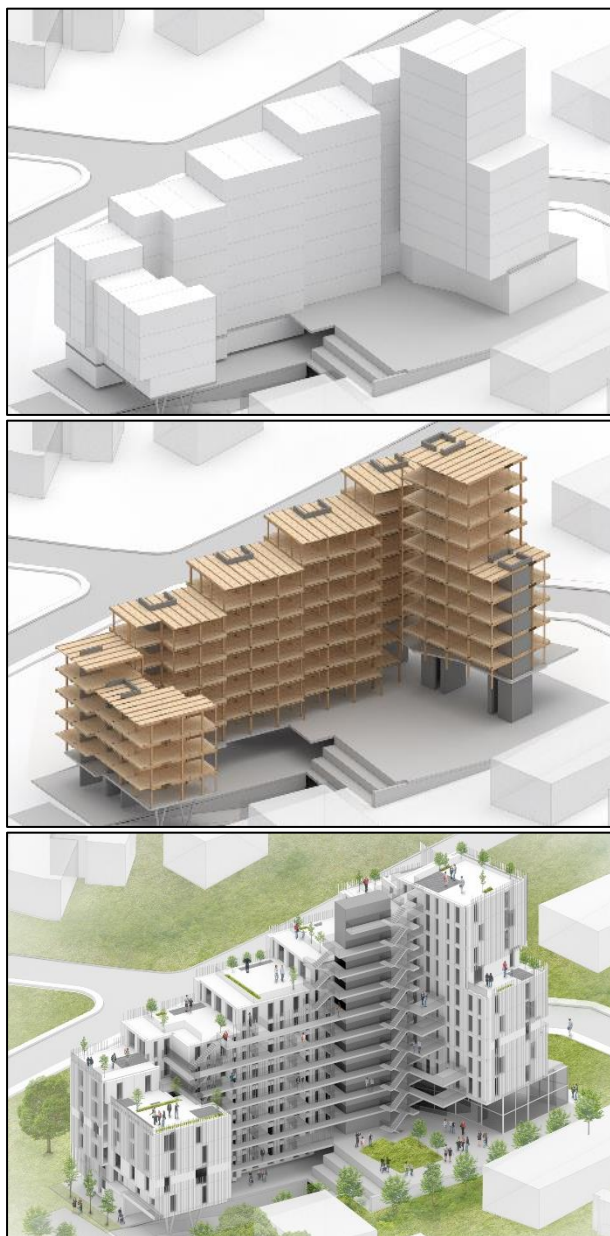
Figure 6. Visualisation of the modular layout (top) and the resulting construction system (bottom) for Corvette Landing. Each panel has a different geometry due to the setbacks, column positions and concrete cores
