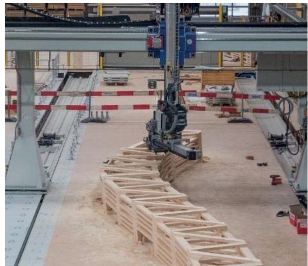
Figure 1. Robotic assembly of large timber trusses for the ETH Zürich Arch_Tec_Lab. Source: ETH Zürich, Apolinarska 2016 [21]
