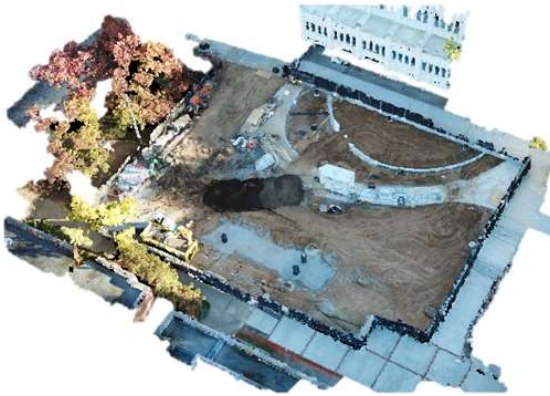
Figure 3. UAV-generated 3D point cloud map of the construction site using image data
