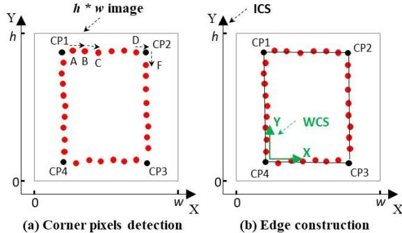
Figure 3. Object shape extraction from a segmented mask
