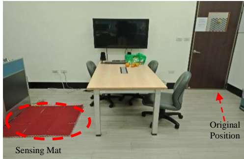
Figure 6. Sensing mat installation positions
