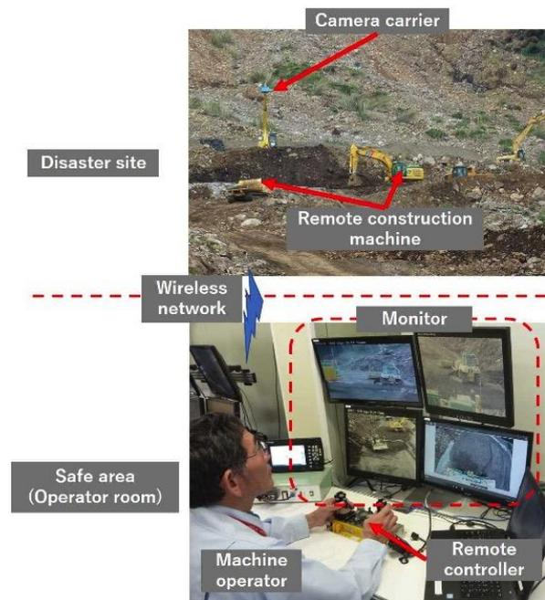
Figure 1. Unmanned construction system using conventional LCD monitors.
