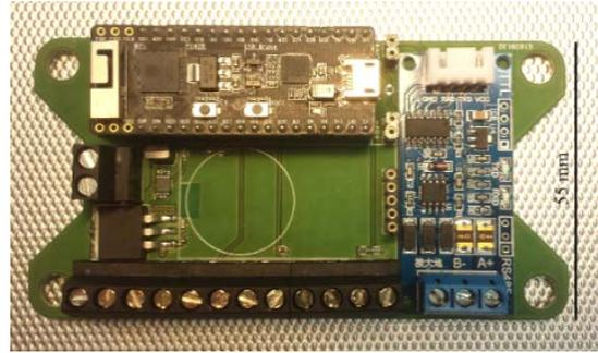
Figure 4. Assembled IoT-gateway PCB prototype from our defined requirements
