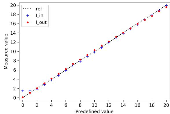
Figure 6. Validation of 0-20 mA input and output
