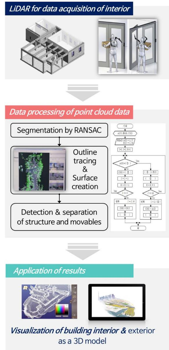
Figure 3. Process for 3D modeling based on point cloud data retrieved by LiDAR
