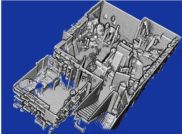
Figure 7. Scanned interior of basement
