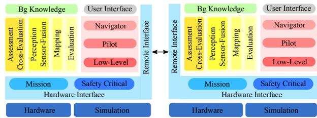
Figure 3. Robot communication using REACTiON remote interfaces.
