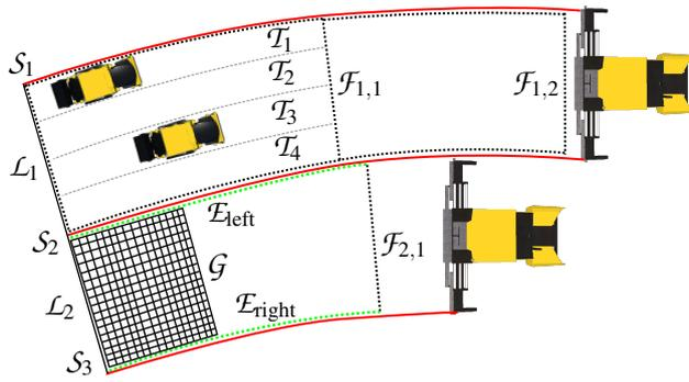
Figure 2. Road  $\mathcal{R}$  with lanes  $\vec{L}$ , seams  $\vec{S}$ , fields  $\vec{F}$ , edges  $\vec{E}$ , grids  $\vec{G}$ , and tracks  $\vec{T}$ .
