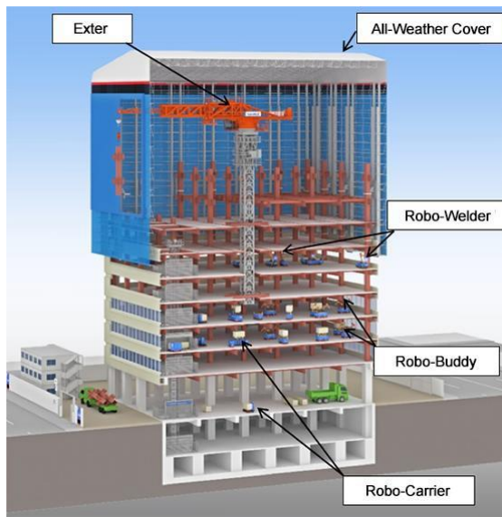
Figure 1. Shimizu Smart Site
