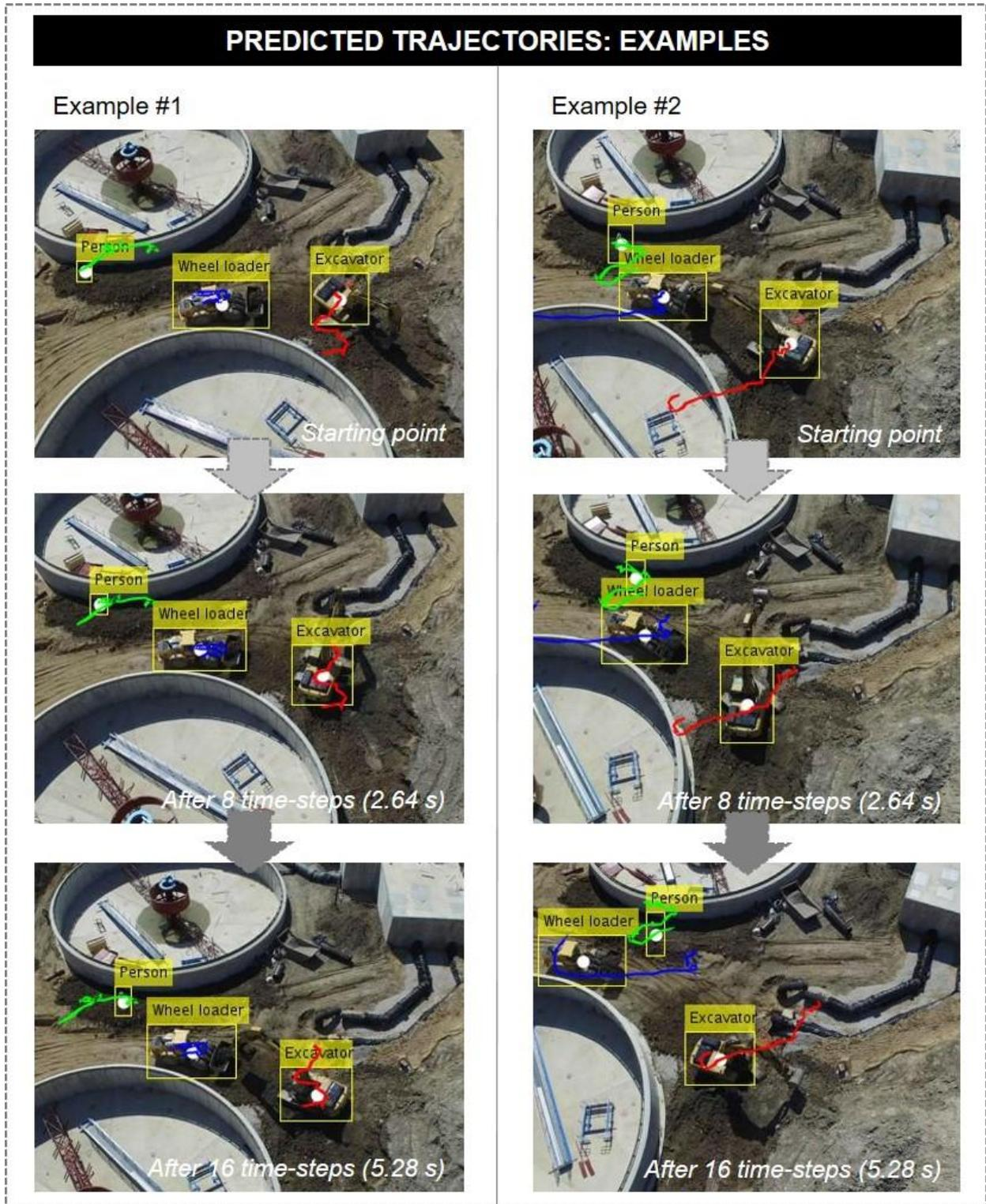
Figure 2. Predicted trajectory vs. ground truth positions
