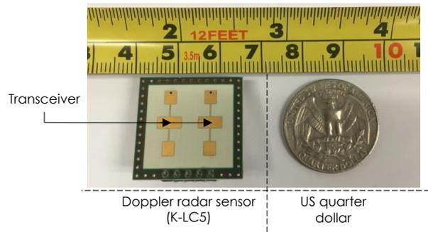
Figure 5. Doppler radar sensor used in this study
