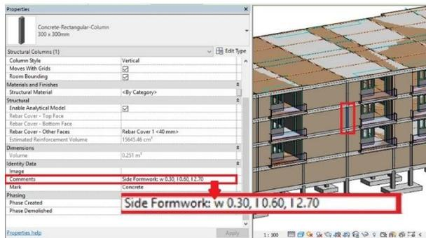
Figure 8. Sample of a formwork combination added to the BIM model
