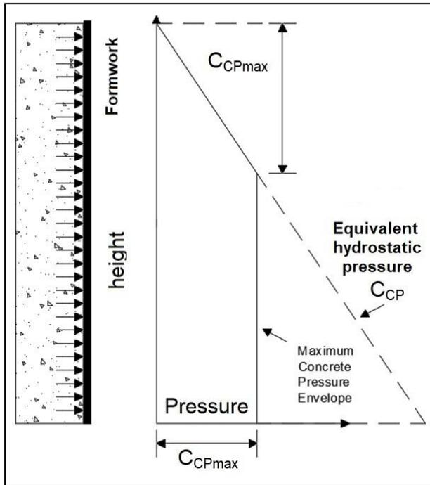
Figure 3. Schematic view of the lateral concrete pressure [15]
