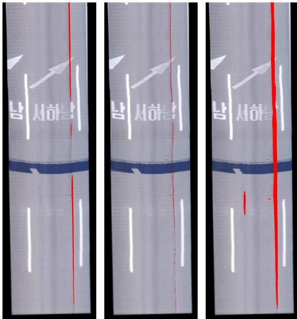
Figure 3. Examples of pavement crack mosaicking results (from left to right: CDQ based method, overwriting method, and accumulating method)
