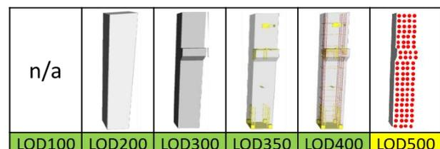
Figure 2. The different LODs of a precast structural column out of the LOD Spec. Guide, extended by a self-made illustration of LOD500.
