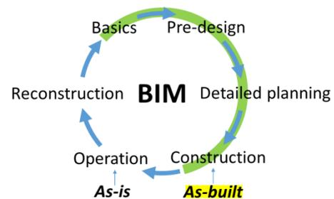
Figure 1. As-is and as-built BIM in lifecycle
