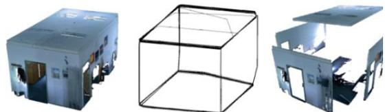
Figure 5. Point cloud segmentation for planar segments. Left: Input point cloud. Center:
